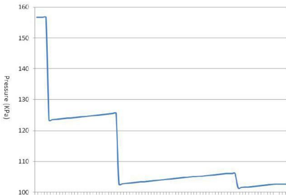
Response of pressurised vessel following stepwise depressurisation
